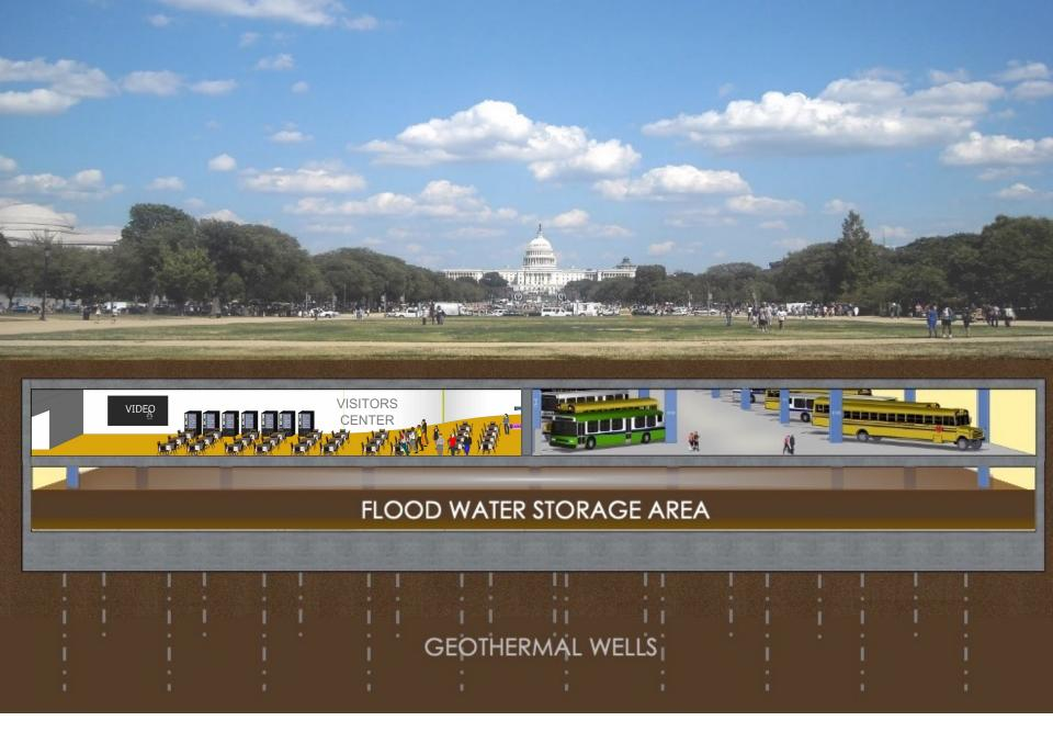
Lower level serves as stormwater reservoir during flood events, after buses are vacated
